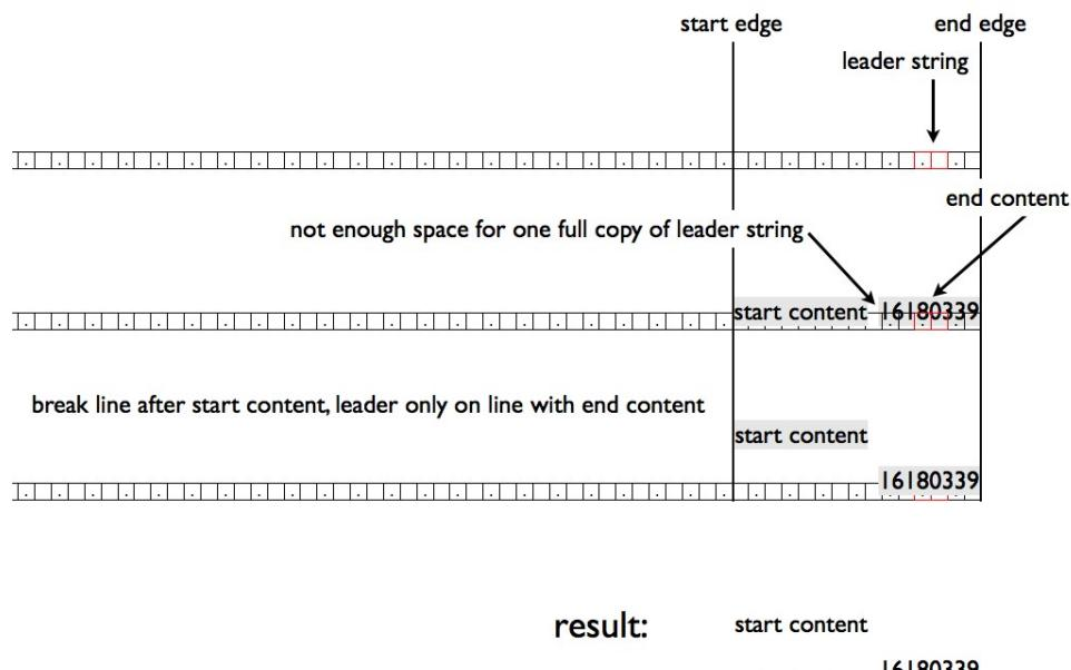
**Figure 2** Procedure for drawing leaders when the content doesn't fit on a single line
